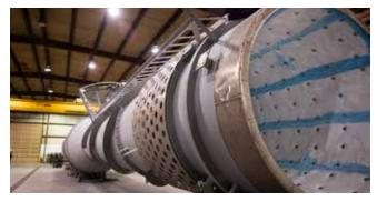
APTIM's subsidiary, LFG Specialties, designed and implemented an ultra-low emission landfill gas flare for a national waste management company to reduce greenhouse gas emissions.
